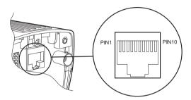
Figure 4. RJ45-10 Connector
